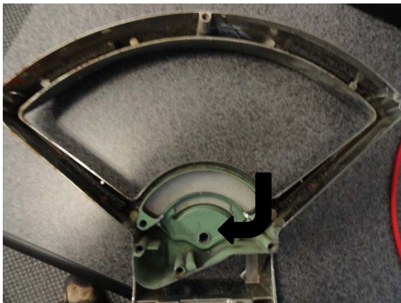
Insert OEM Gear Indicator Assembly ( With Pointer Removed ) Over Window Lens
